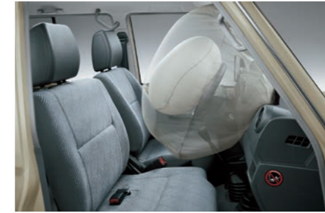
Front-seat dual SRS* airbags supplement the restraining action of seatbelts to provide further protection in the event of a front-end collision (Optional)
