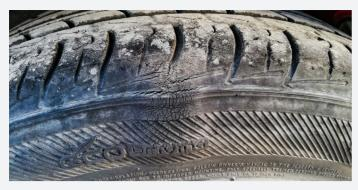
The tire tread should be worn evenly and all four should match. Uneven tread or extra wear on a few of the tires often means poor alignment, which can be a symptom of steering, suspension, or frame issues. A poorly aligned car will pull to the right or left when driving.
